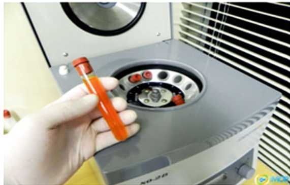
Fig. 9 Plasma tube with ACD before the 2nd centrifugation at 1,800 rpm, for 10 min
